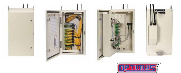
The pole/wall mounted Optimus Cabinet Fiber Hub is a powder coated aluminum cabinet designed for centralized split points in a PON network. The 72, 96, 144, 288, and 432 fiber termination choices allow operators to scale the cabinet cost to their network design.
